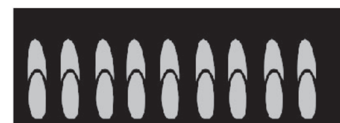
(A) Soft blue flames - Normal for natural gas
