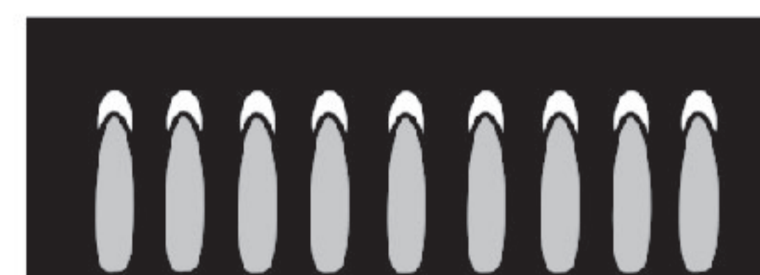
(B) Yellow tips on outer cones - Normal for ULPG gas
