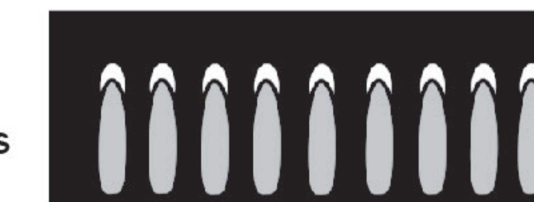
(B) Yellow tips on outer cones - Normal for ULPG gas
