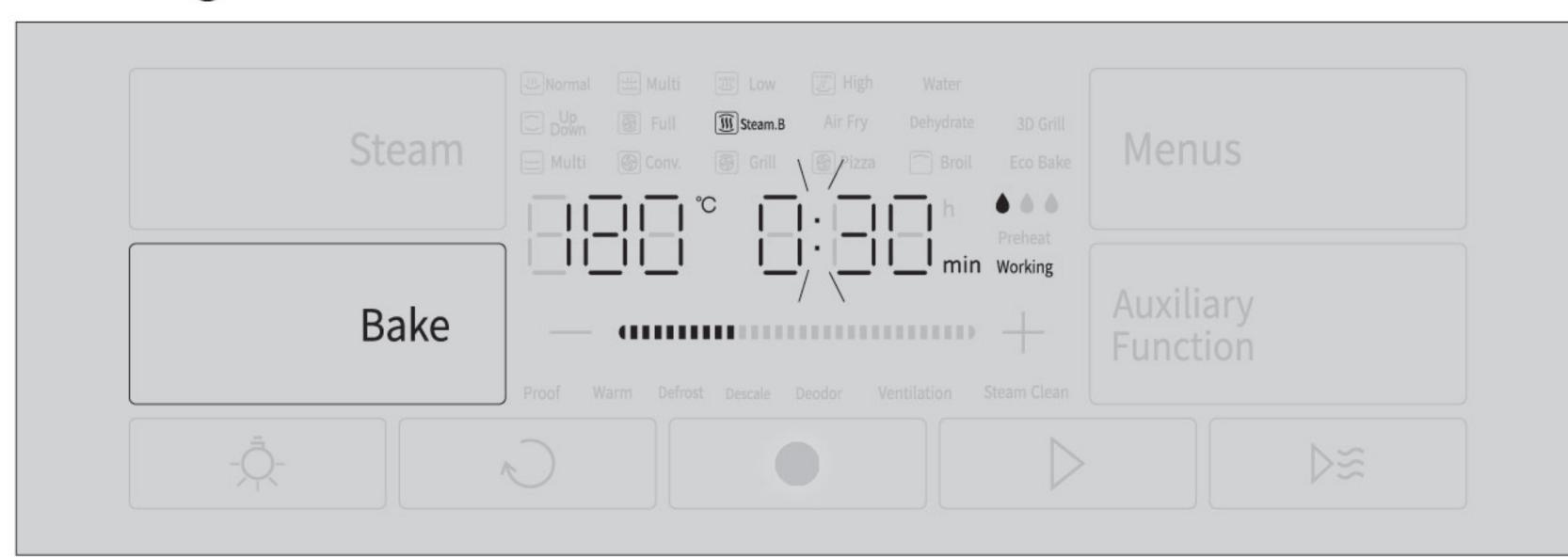
5. **Cooking finished.** The countdown reaches zero, the work is completed, with ten buzzers given.
