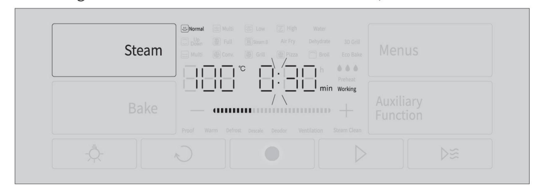
4. Cooking finished. The countdown reaches zero, the work is completed, with ten buzzers given.
