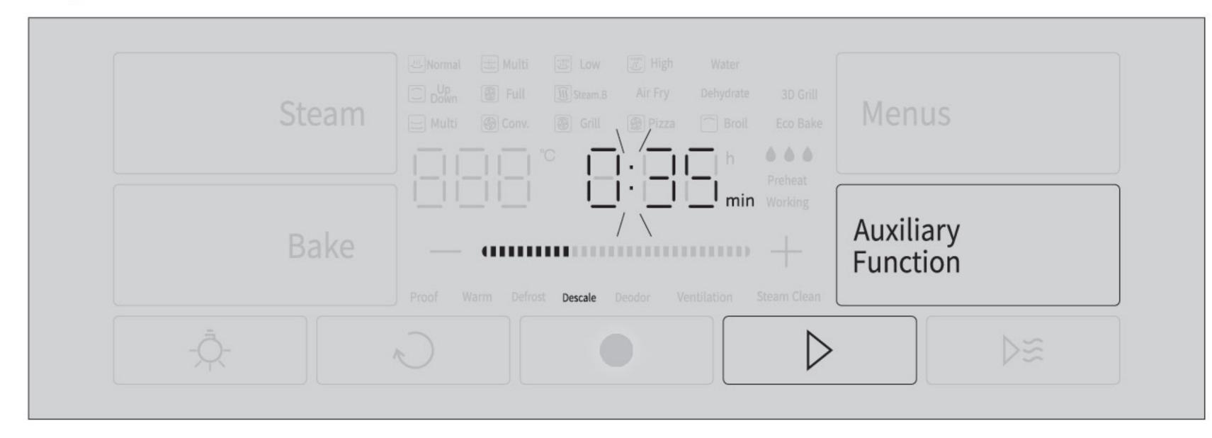
4. Descaling is completed. After the work is completed, the countdown reaches zero, with ten buzzers given.
