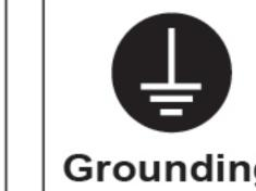
The socket must be equipped with a reliable grounding wire to ensure Grounding safety. Do not connect the grounding wire to the gas pipe, water pipe, lightning rod and telephone line. Imperfect grounding may cause electric shock or other accidents.
