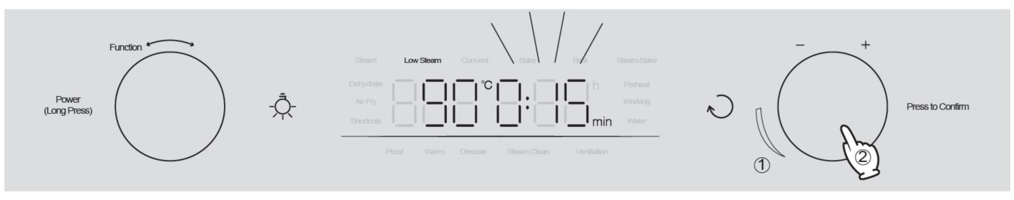
4. **Preheat.**When the oven starts to preheat, the real-time temperature is displayed.
