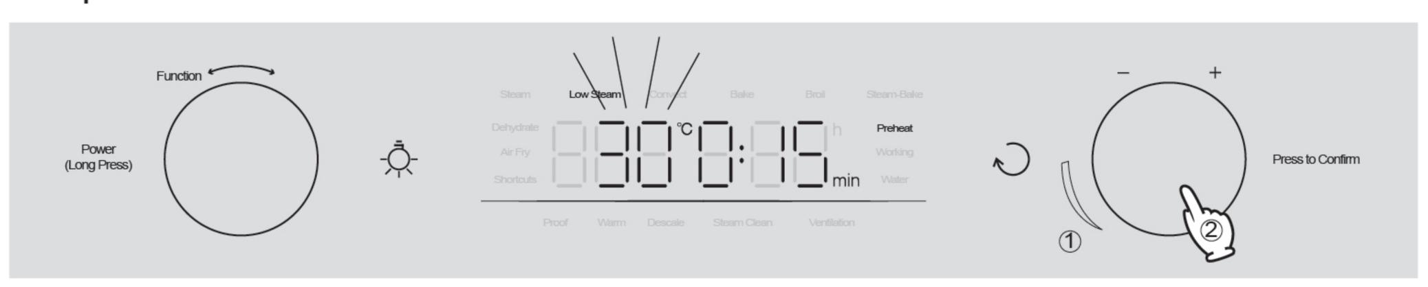
2. **Modify time parameters.**Turn Knob 2 to set time and confirm the modification with a short press of Knob 2.
