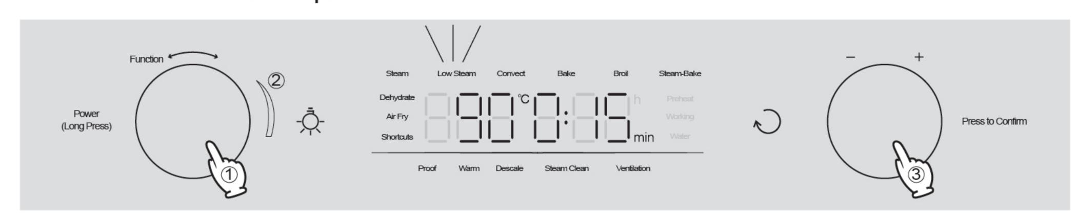
2. **Set cooking temperature.** Turn Knob 2 to set temperature and confirm the temperature with a short press of Knob 2.
