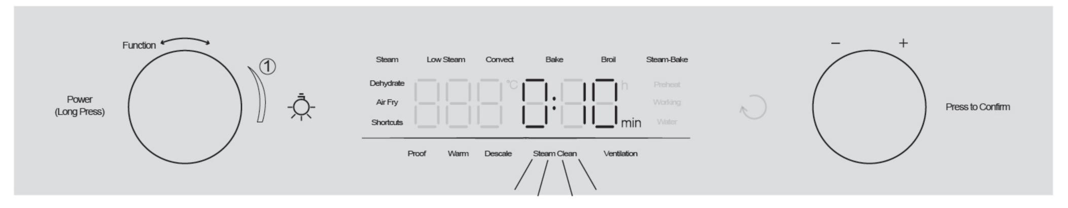
2. **In operation.** Turn Knob 2 to start working, and time starts counting down. Press button to exit.
