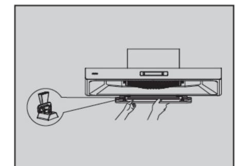
6. First, grasp the front edge of the wing plate with both hands, flip it downward to make the wing plate claw detach, then flip it downward by a certain angle, and finally take out the wing plate with both hands holding it smoothly.
