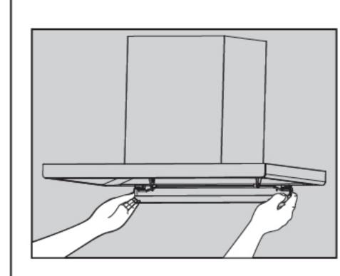
7. Hold both ends of the grease cup with both hands. Remove it straight out while maintaining horizontal alignment to drain accumulated grease. Immerse both the grease cup and flow straightener plate in warm water with neutral detergent, then clean using a soft brush.
