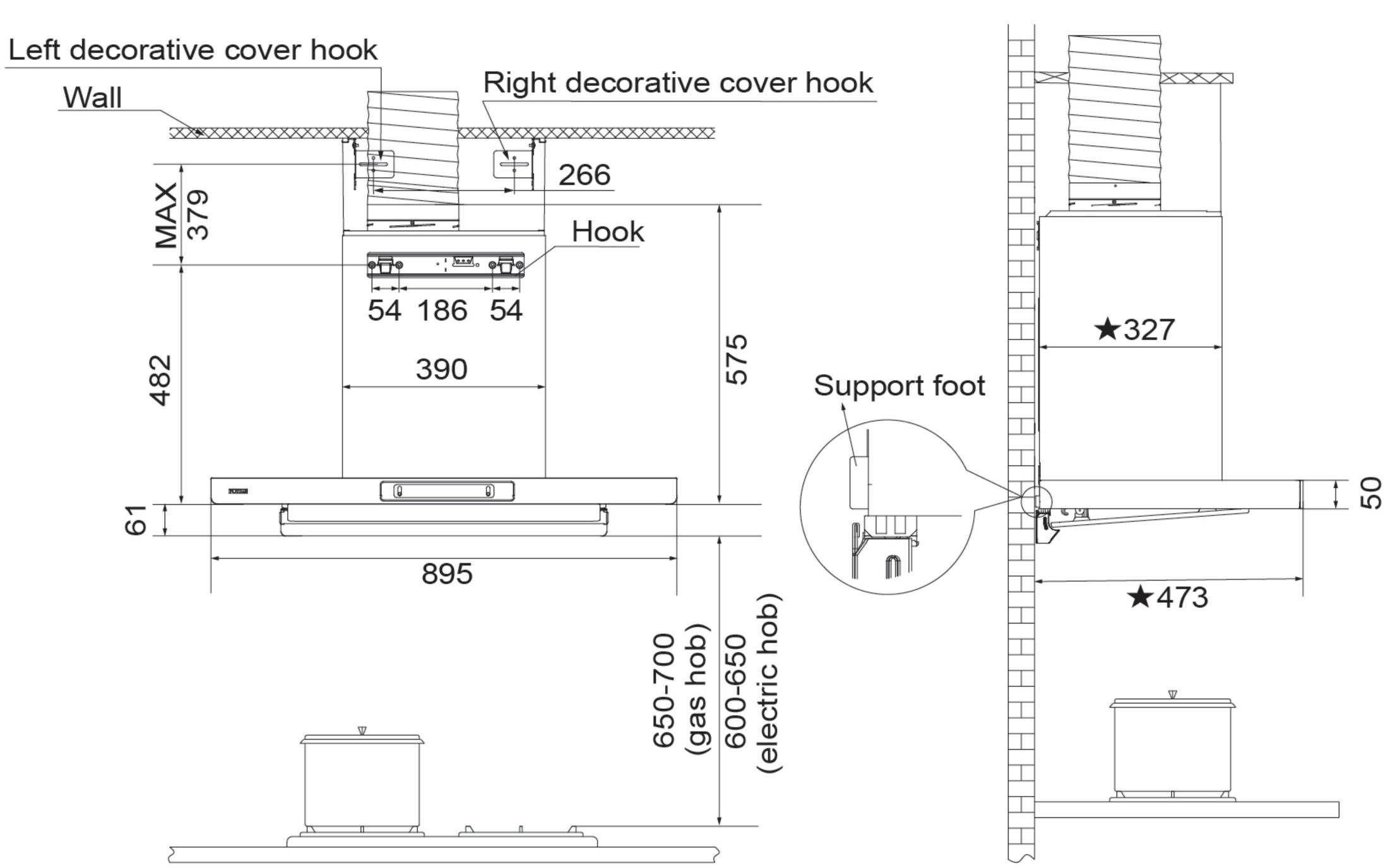
EMG9063-G Installation diagram (★ is the distance from the wall)
