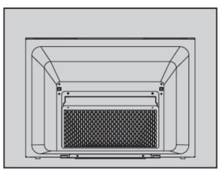
Drag the oil screen with the left hand and loosen the two screws that secure the oil screen with a Phillips screwdriver in the right hand to remove the oil screen.
