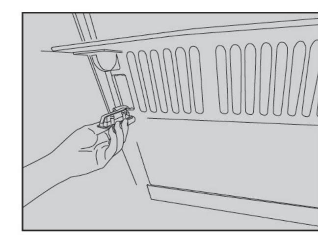
10. Take apart the connecting line of lamp, replace the whole LED lamp.
