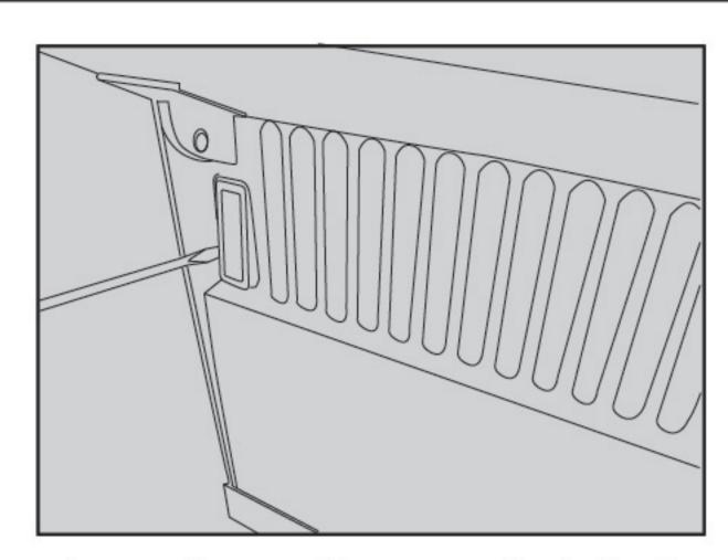
9. Insert the edge of lamp slightly by small straight screwdriver, pry downward and take out lamp components.
