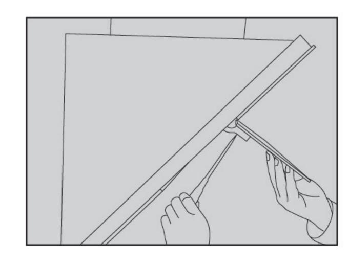
8. Unscrew 4 setting screws on the Smoke battle, slightly push upward the glass and take down the Smoke battle.
