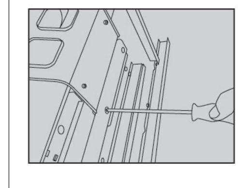
9. Use the cross screwdriver to open the screws of the connecting rod (two on both sides respectively, and disassemble the lifting poker;
