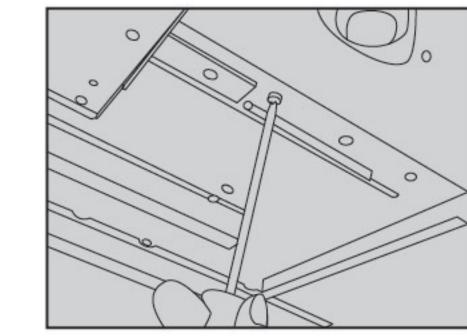
10. Use the cross screwdriver to open the five screws in the fan frame (one on both sides respectively, Figure 16;
