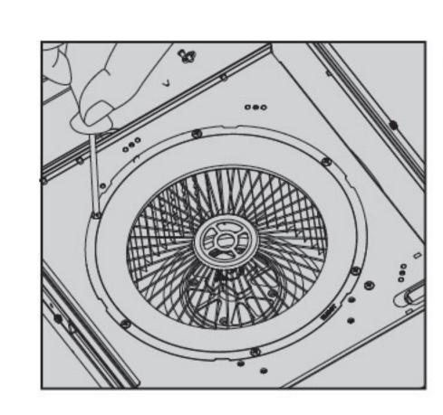
. Use the cross screwdriver to open the screws on the air inlet ring.
