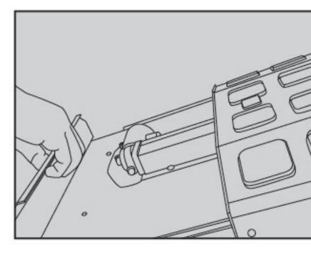
three on the top, open the four screws on both sides, open the screw on the fan cover, and disassemble the fan cover plate.
