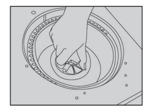
12. Screw down the locknuts clockwise, and take down the impeller.
