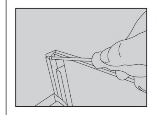
8. Use the cross screwdriver to open the two screws used to fix the fan outer cover, and take down the fan outer cover and the trim cover.
