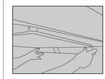
The two ends of the oil cup shall be held by both hands, maintain the horizontal level of the oil
