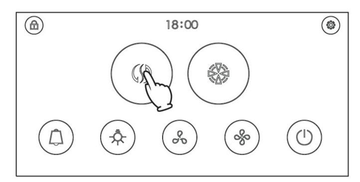
Press (§) key to enter Kitchen Air Steward interface. The range hood can detect air quality automatically.
