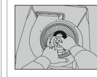
13. Screw off the locknut clockwisely, Take out the impeller.
