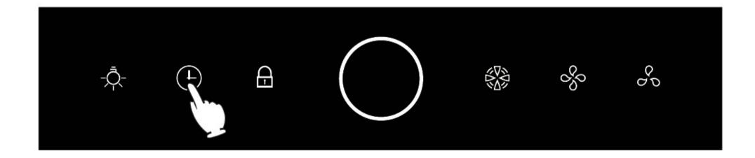
If you press when the range hood is working or on standby, it also will be turned off automatically after 2 minutes, if you need to cancel the delay, press any key.
