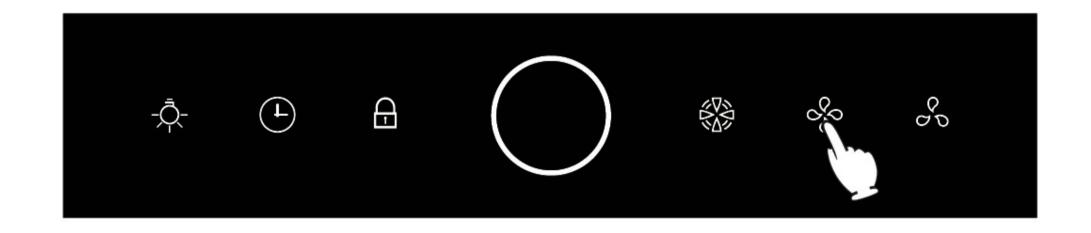
You press the % key, the light indicator will show "on", the relevant working condition is "middle power". Press the % key again, the light indicator will show "off", the relevant working condition is "off".
