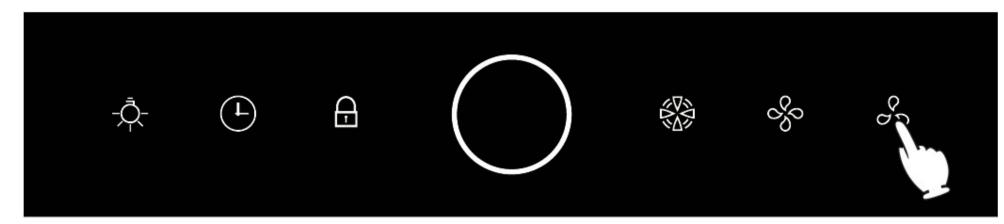
You press the & key, the light indicator will show "on", the relevant working condition is "weak power". Press the & key again, the light indicator will show "off", the relevant working condition is "off".
