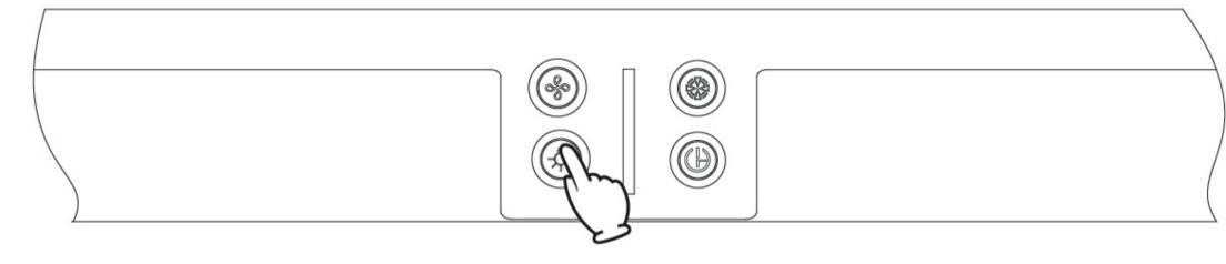
Press the "-\(\bar{\pi}\)-"button, the light is turned on, and press the button again, the light is off.
