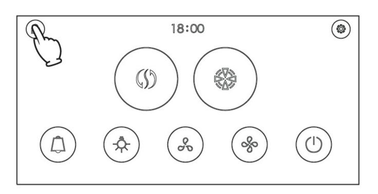
Press 🗎 key to enter the panel lock interface. Slide to unlock.
