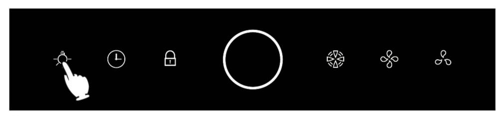
Press the 🖒 key, the light is turned on, and press the key again, the light is off.
