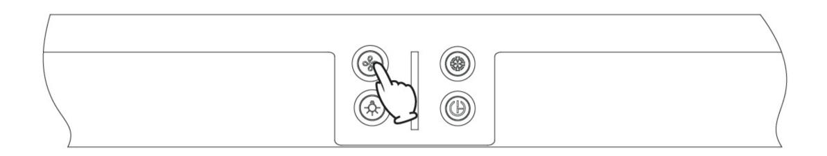
Touch the button %, the motor shall be started; the indicator lighting of % button is fully-lighting, and the range hood is running at the strong grade; then touch the button again, the indicator lighting of % button is semi-lighting, the range hood is running at weak grade, touch again, the function is turned off.
