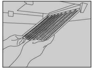
7. Firstly, hold the front end of ring suction plate with both hands, turn downwards, so that the fastener of ring suction plate is out of place,
