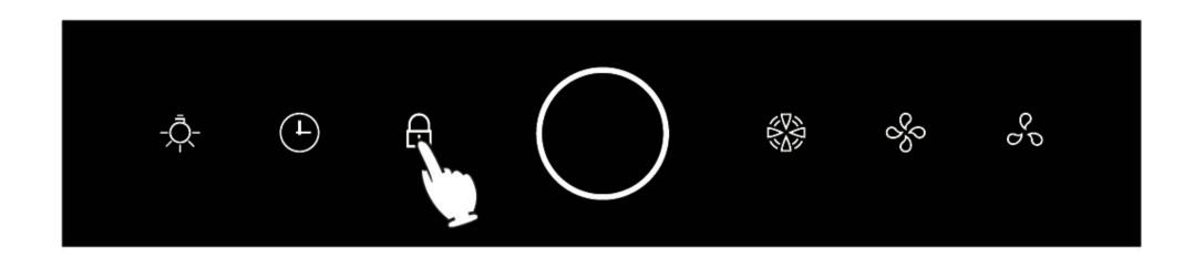
During working state or standby mode, Press the key at least with 3 seconds, the range hood beeps once, flashes on, all keys will be locked, and clicks invalid, the range hood will emits a beep; then press at least with 3 seconds, the screenlock function is canceled and resume.
