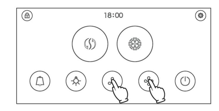
Press & key, the draught fan runs less powerfully. Press it again and it stops. Press & key, the draught fan runs powerfully. Press it again and it stops.
