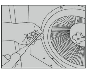
10. Unscrew the screws fixing on the air input ring, and remove the air input ring.
