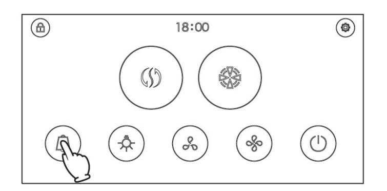
Press key to enter the alarm clock setting interface and set the countdown alarm clock. Prompt tone will be heard when time is up. The prompt tone lasts for 2 minutes (touch any key to stop the prompt tone) and it will stop automatically after 2 minutes.
