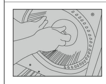
12. Unscrew the locknut in clockwise direction, and remove the vane.
