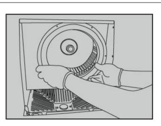
11. loosen the screw, take off the air inlet.
