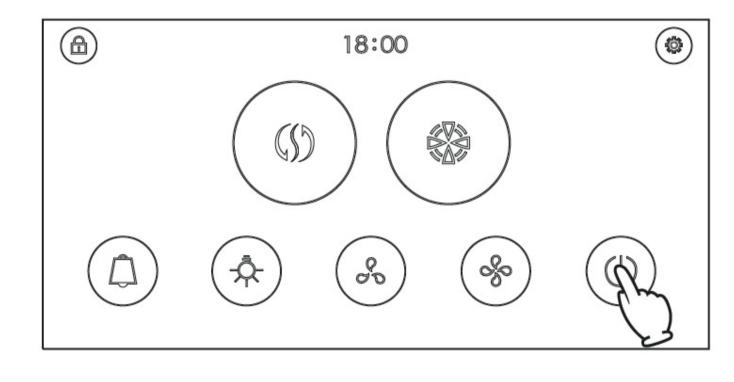
Press () key and the device is turned off. (If "delay shutdown" is set, this function will be implemented.) All functions are immediately turned off to enter the black screen or clock screensaver interface. Click anywhere on the screen again to enter the main interface.
