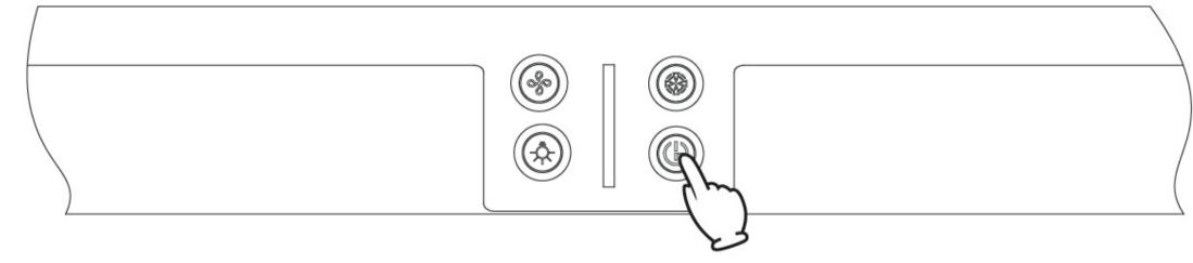
When (b) is touched, the range hood will standby for operation. If there is no operation on stand it will be turned off automatically.
